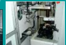
The grippers for transferring crystallisation plates between the Homebase vault and the Veeco imager
